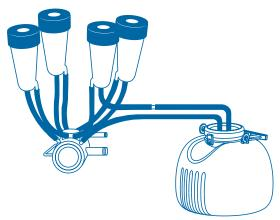
**2.** Connect the Quartermilker to the claw by disconnecting the required inflation and joining it to the plastic connector on the Quartermilker tube. The other Quartermilker tube (the one attached to the lid at the safety valve) is then connected to the milking claw.
