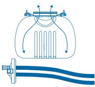
After cleaning, drain all sanitizing solutions from the bowl and lid assembly, and leave open to air dry. Do not disconnect the rubber hoses from the lid more often than necessary. Occasionally soak the whole assembly in acid solution and use a brush to thoroughly remove any milk and mineral deposits from the bowl, lid and all tubes.
