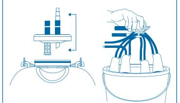
**3.** The rubber tube without the connector should always be fitted to the side of the lid with the safety valve. If the valve becomes close while attaching the cluster to the cow, squeezing this tube temporarily can cause the valve to open again.
