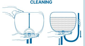
Fill the bowl of the Quartermilker with warm water and detergent. Attach the lid assembly and agitate thoroughly while holding upside down. Lift the rubber tubes alternately to syphon air and wash liquid through.
