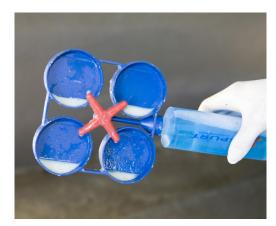
**Step 3:** Tilt the paddle to a 45 degree angle and pour off excess milk down to line in bottom of paddle; this will leave equal amounts in each tray.
