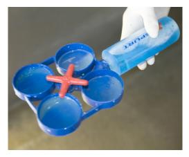
**Step 4:** Add equal parts of RMT reagent to milk (squeeze) and mix by swirling or rocking the paddle for 10-15 seconds.
