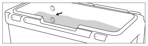
If using the automatic water supply option, connect the water supply using the quick connector and the adaptor.
