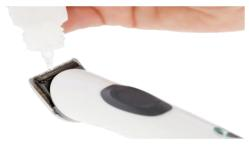
Repeat oiling every 5-10 minutes during operation. This prevents the clipping head becoming hot and being overloaded. It would then become duller sooner and then must be replaced sooner.
