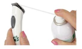
An oil spray with a small tube attachment is well suited for cleaning and oiling between the blades.
