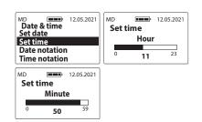
5.6 c) **Date notation** – to change the format of date display, go to **Main menu / Settings / Date & time / Date notation**, then use the or key to select the appropriate option and confirm with the OK key, e.g.
