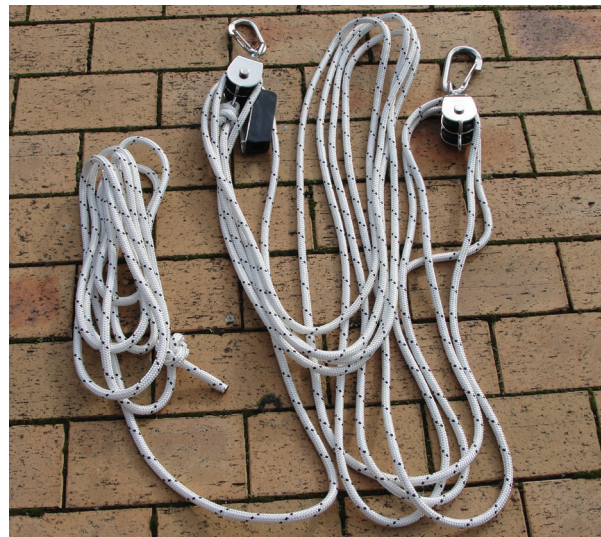
Another type of locking pulley. No storage knot tied in the photo. Lots of rope to potentially tangle!
