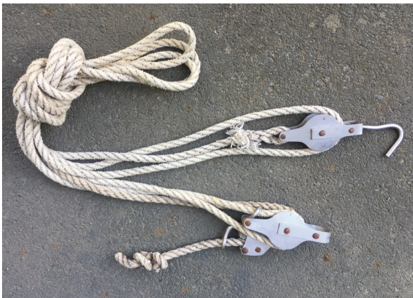
3:1 locking pulley above. This is the one I most often use.
