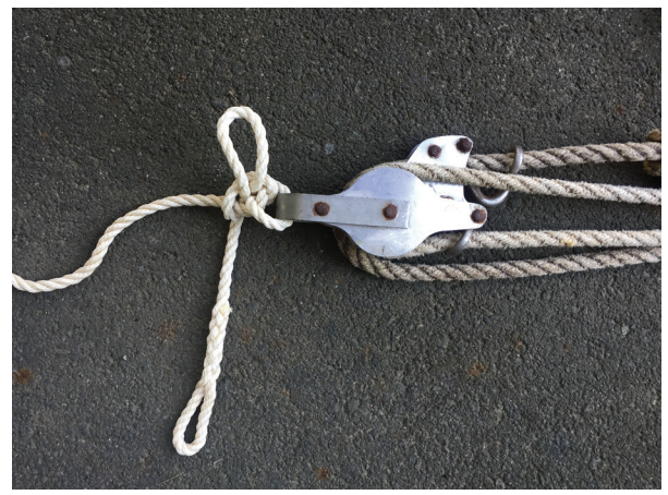
I use 2 hitches with a loop in the second one as shown above.
